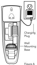
**6.** Slide the Charging Base into place making sure the cord exits through one of the slots.
